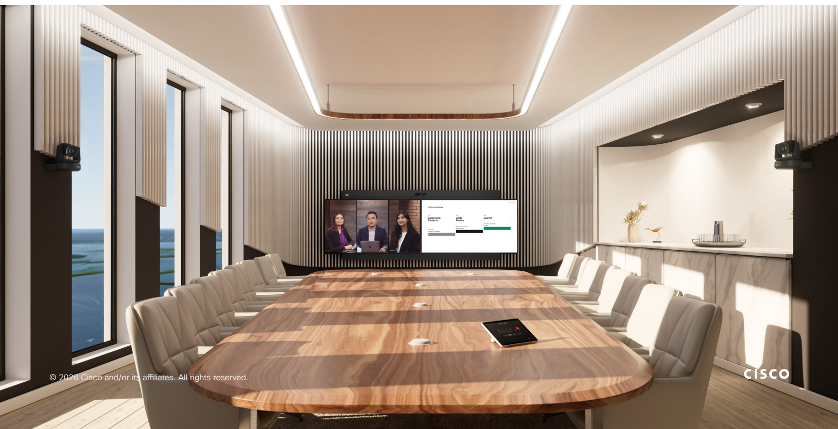
Figure 2: Room Vision PTZ cameras deployed in a boardroom combined with a Room Kit EQX to support the inclusive cross-view experience.
